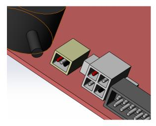
If the LED port is not receiving at least 4.5v, then there is a fault in the board. The board must be replaced.
