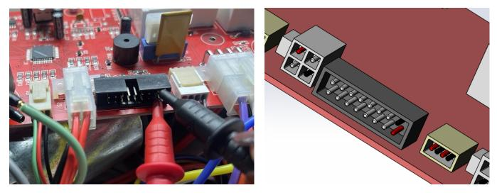
If the LCD port is not receiving at least **4.5v**, then there is a fault in the board. The board must be replaced.
