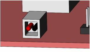
If the PCB is not receiving at least **26v**, the charging beak or charging dock is broken. See charging dock troubleshooting guide to determine any faults with the dock. If none arise, then replace the charging beak.
