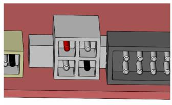
If the Port is not receiving at least **26v**, then the power is being lost in between the charging port and the main power port, this means that the PCB is broken and needs replacement.
