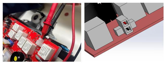
If the drive motor port is not receiving at least 18v, then there is a fault in the board. The board must be replaced.
